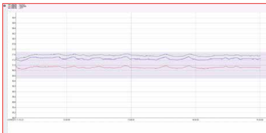
Graphic of temperature stability and homogeneity, obtained with three PT 100 probes equidistant at the centre of the chamber
